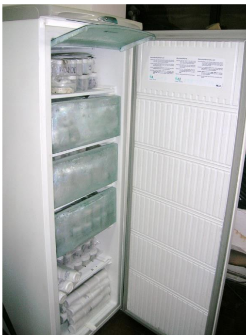
Figura 1. Banco base original del BNGP FCA-UNC, envases tapa a rosca, freezer - 18°C.
