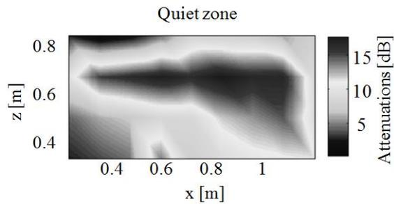
Fig. 8. Quiet zone in the area defined by error sensors and secondary sources.
