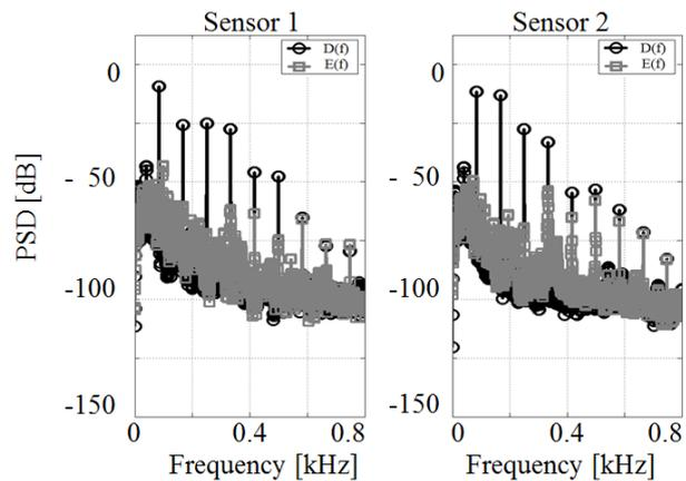
Fig. 7. Error signals PSD with ANC system off and on (D(f) and E(f)).
