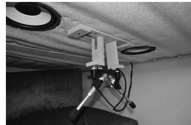
Fig. 3. Secondary sources and error sensors inside the enclosure for 2x2 ANC system.
