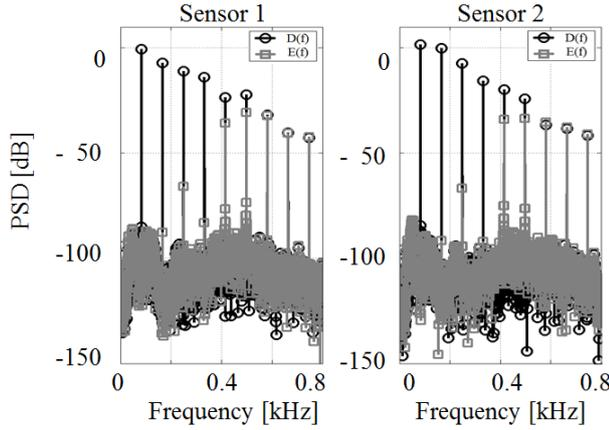
Fig. 4. PSD of error signals in simulations for 2x2 ANC system off and on ( $D(f)$  and  $E(f)$ ).
