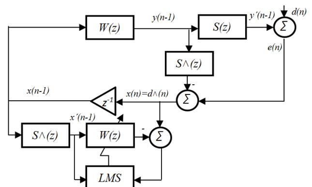
Fig. 1. Single channel MFxLMS algorithm diagram.
