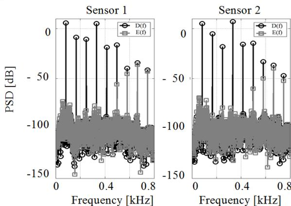
Fig. 2. PSD of error signals in simulations for 4x2 ANC system off and on (D(f) and E(f)).
