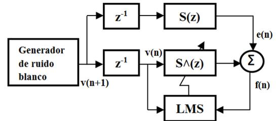
Fig. 5. Secondary paths identification scheme
